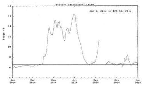
Figure 1. Stages of Lake Pepin at Lake City during 2014. Source: Real time data link, www. mvp-wc.usace.army.mil. Used with the permission of the U. S. Army Corps of Engineers.
