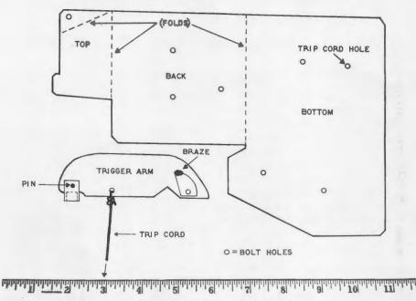
Figure 2. Carriage diagram (upper) and trigger arm (lower left). Scale in inches.
