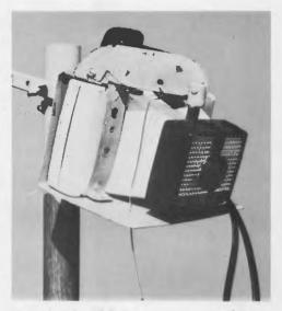
Figure 1. Polaroid Swinger camera mounted in carriage and attached to tubing section.
